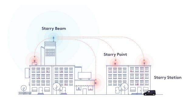
Caption: How Starry Internet Works. Starry Beam (network node) communicates to Starry Points (located on your apartment building or home) located within a 2km radius using millimeter waves. Starry Point then connects to your Starry Station WiFi hub using in-building wiring to deliver whole-home, ultra-fast, reliable broadband.
